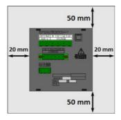
Use the enclosed fixing clips to fix the UMD 97 in the control panel. Place them on the side of the device and fasten them with a screwdriver.
