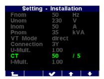
Once you have made the necessary settings, confirm them with button 3 and return to the main menu by pushing button 1 repeatedly. Confirm the subsequent query with button 2.
