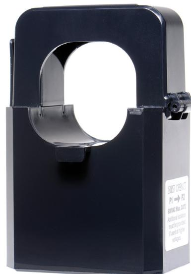
These hinged core transformers provide a secondary output current of 1 A, 5 A and 100 mA, respectively, based on the recorded nominal input currents, which makes cable lengths non-critical. It can be used for electricity meters and power meters in power distribution systems, control panels, switchgear and other equipment.
